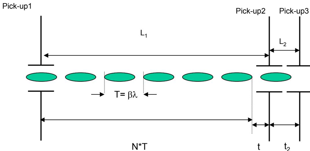
$$\frac{\Delta\beta}{\beta} = \sqrt{\left(\frac{\Delta L}{L}\right)^2 + \left(\frac{\Delta t}{NT + t}\right)^2}$$
