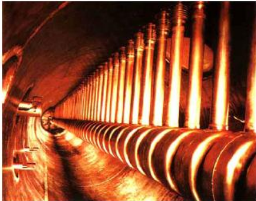
Saturne DTL (Saclay) : -> 20 MeV, 200 MHz
