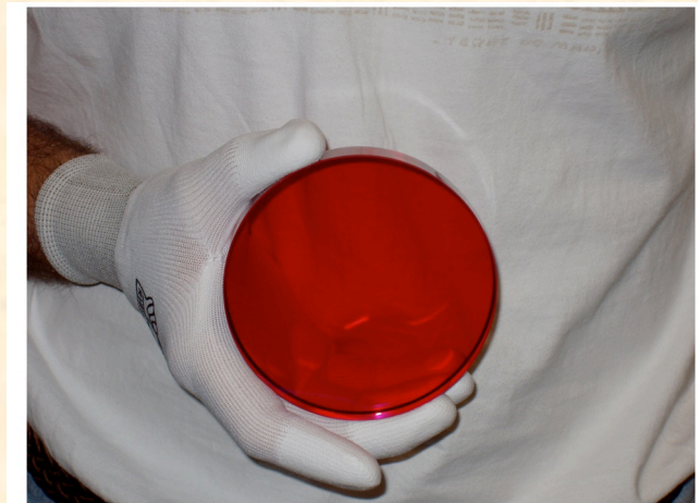
Ti:Sa crystal of the high-energy amplifier (Crystal Systems, Salem)
