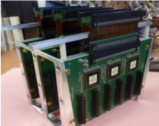
6 FM EC-ASIC in mechanical structure
