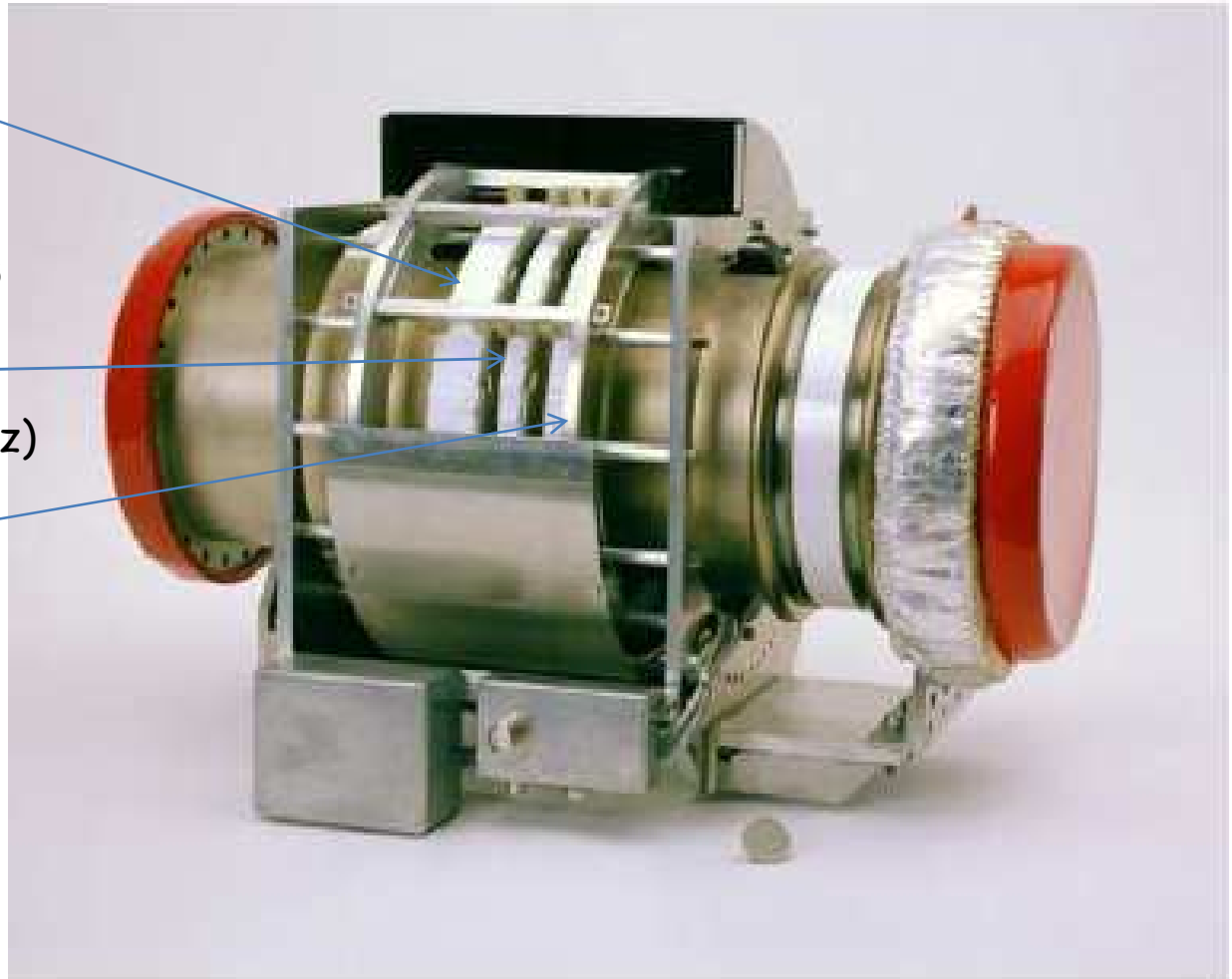
DC and AC Beam current transformer à GSI
