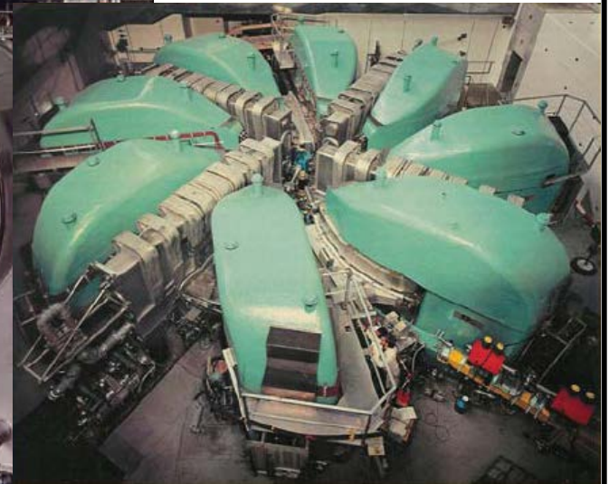
Cyclotron PSI (p, 590 MeV, 2mA, 50.6 MHz)
