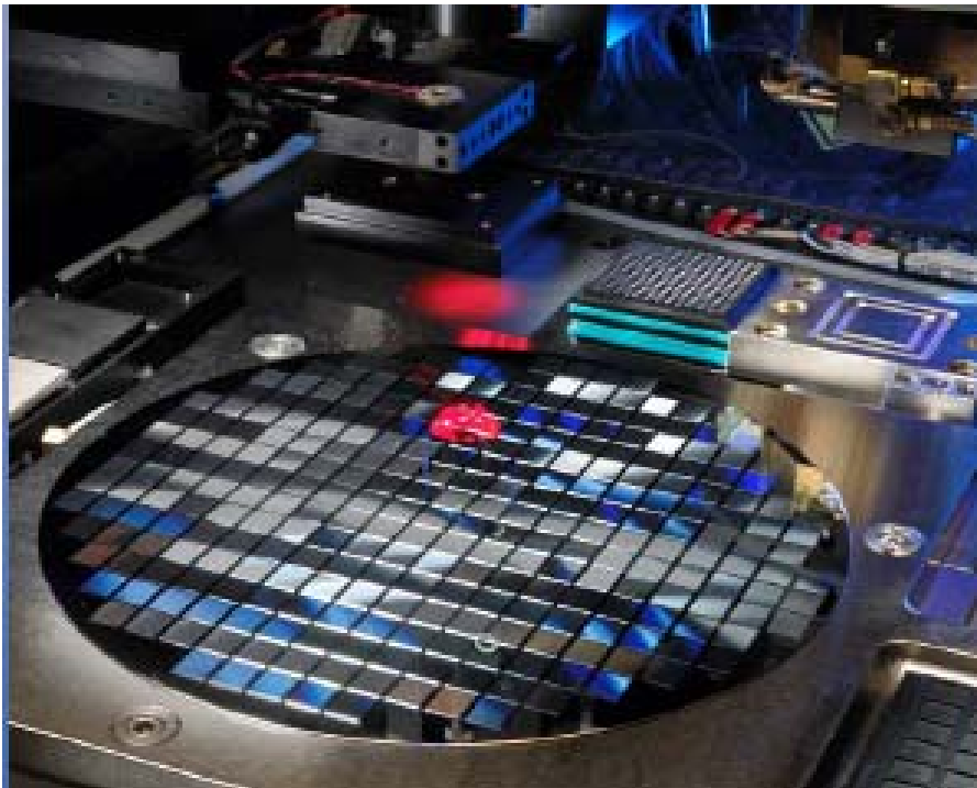
Die to Wafer alignment and placement
