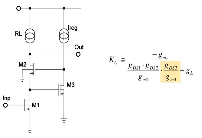
Cascode transistor controlled with common source amplifier
