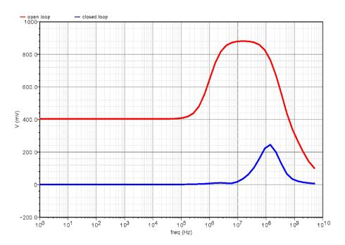
Power supply disturbance (1V) seen at cascode output working in open loop configuration (red) and in transimpedance preamplifier (blue). 130nm version of front end.
