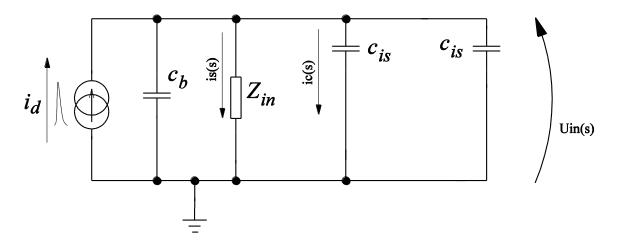
In this case we assume that input of the preamplifier is loaded with  $c_b$  and two  $c_{is}$  capacitances (neglecting input impedances of the neighbors). Using Kirchhoff law one can write:
