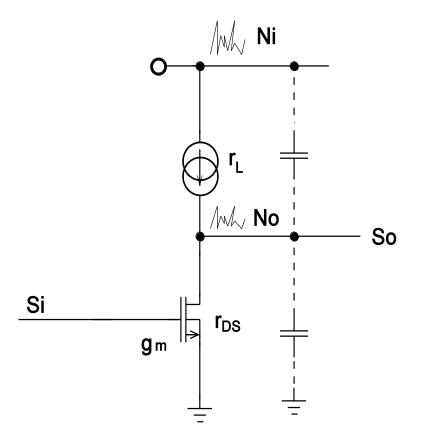
$$K_U = \frac{So}{Si} = g_m \cdot \left( r_L \parallel r_{DS} \right)$$
