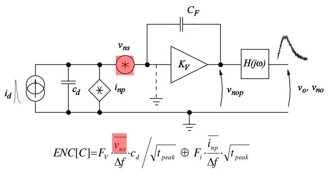
$$\frac{\overline{v_{n \text{ thermal}}}}{\Delta f} = \sqrt{\frac{4 \cdot k \cdot T \cdot n \cdot \gamma}{g_m}}$$
