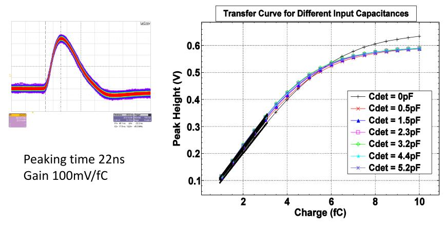
Good linearity up to 4fC (400mV signal range) Dynamic range up to 6fC (limit set by the bias of the differential stage). Good agreement with simulation  $\rightarrow$  the same figures for 130nm version
