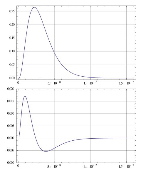
Kv=83dB,  $\tau_{p0}$  =200ns, GBP=1GHz <sup>\*)</sup> Detector;  $c_{is}$ =7pF,  $c_{b}$ =4pF (ATLAS SCT)
