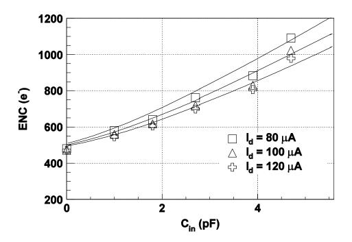
Markers are measurement points, lines are theoretical fit with excess noise set to **3**!.
