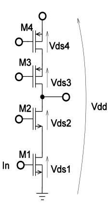
□ All, four, transistors must be in the saturation ( $V_{DS} \ge V_{GS}$ -  $V_T$ )
