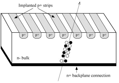
electron-hole pair created along particle track
