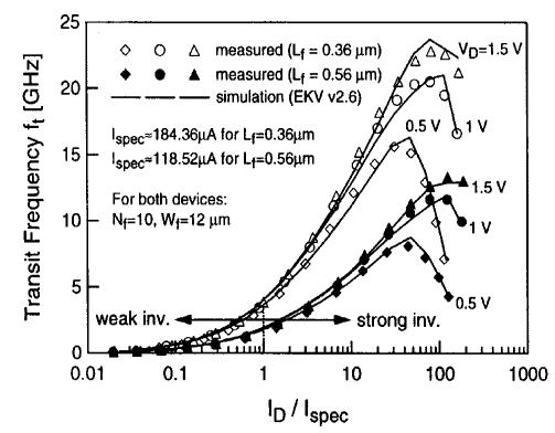
Transit frequency ft as a function of inversion order for 250nm CMOS technology \* For devices biased in weak inversion we never obtain highest possible speed of a given technology
