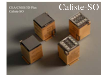
Micro gamma-camera for Solar Orbiter (ESA Mission)
