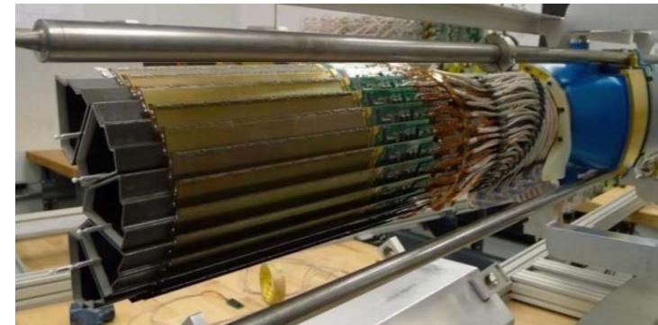
2 layers, radius: 2.8 & 8 cm, 40 ladders, 400 sensors, 0.15 m 2
