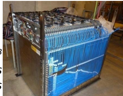
Demonstrator, 1 m 3 40 layers 400 000 Channels
