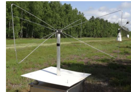
Butterfly Antenna, 2.2 x 1.5 m Codalema @ Nancay - France
