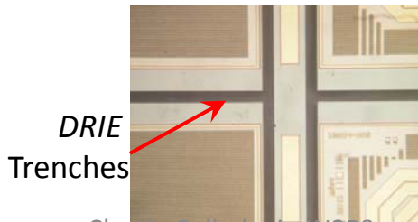
Wafer Scribe Lines pre-diced with DRIE AMS courtesy
