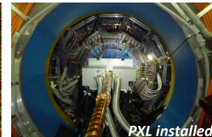
2 layers, radius: 2.8 & 8 cm, 40 ladders, 400 sensors, 0.15 m 2
