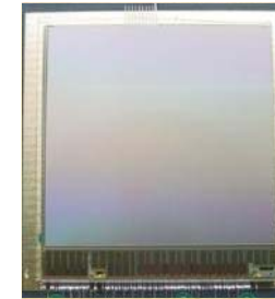
Mimosa 28, ~4 cm 2 , 0.35 μm 2-well CIS, Hres epi layer
