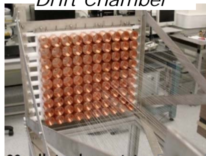
90-cells tracker prototype Manchester-UK courtesy
